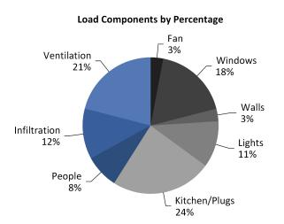
Further, as the unit sensible loads have been reduced, the fresh air loads have stayed constant, if not increased. As a result, the fresh air component is now a much greater percentage of the overall load that must be addressed. The chart above illustrates that that over 40% of a typical apartment load has a latent load component.
